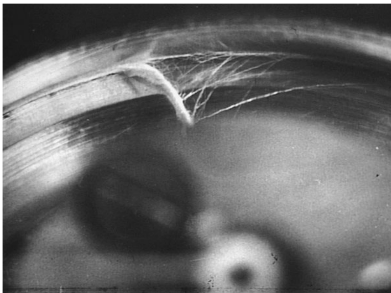
FIGURE 6.45 Wrapper fiber formation.
